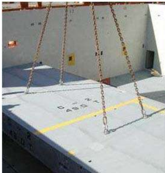
Figure 10 Tweendeck lift-away hatch covers
