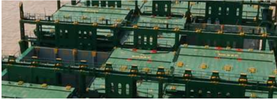
Figure 5 Lift-away hatch covers
